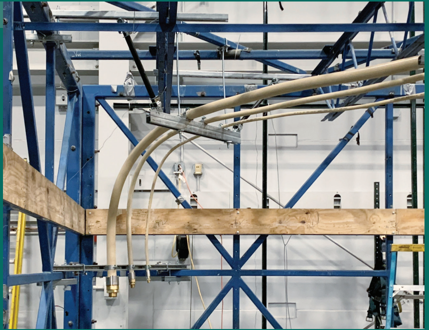
MediTrac® CMT in seismic test rig.
